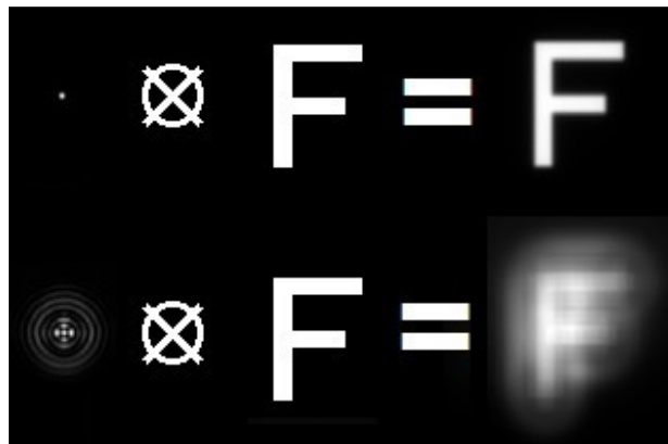
Figure 2.3. Convolution operation: The first situation shows a perfect version of a letter "F" being convoluted with a diffraction limited PSF yielding a slightly blurred letter "F". In the second situation the letter "F" is blurred, point by point by the PSF, to produce a simulation of the blurred image.
