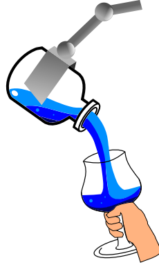
Figure 4.2: Cooperative tasks in which the robot has to pour beverage into the person's cup. Since the cup may be tilted, it is likely that the hand holding the bottle will have to be rotated by angles near to \pi rad.
